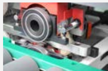
Trimming unit adjustment through the counter convenience and quickly
