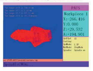
At this moment, the user is allowed to adjust the position of X, Y Z and A axis. The system default manual motion mode is **STEP**. So that user can fine adjust each axis distance (A axis moves by angle). Machine moves one low or high speed grid distance every step.
