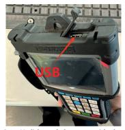
1) Directly import the processing file into U disk, and then run with the U disk inserting in the controller. Press "key, screen shows:
