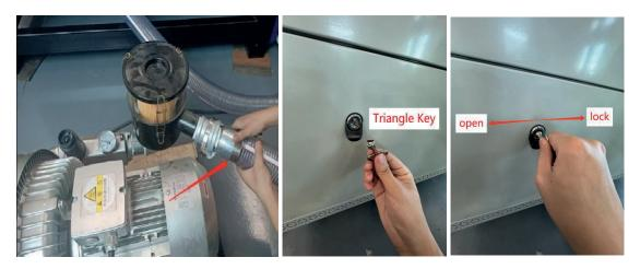
Open the cover of the motor and connect it to the power supply, and connect the other end to the wiring of the vacuum pump controlled by the engraving machine.
