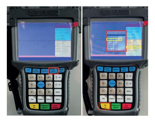
The spindle will move to the tool library for switching according to the selected tool (the tools that come with the machine must be installed according to your needs. We recommend placing commonly used tools in tool holder No. 1. If used in combination,
