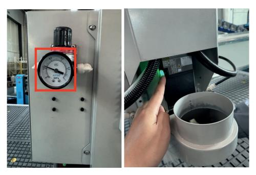
The air pressure should be 0.2-0.4MPa and should not be too high or too low. Press the green manual tool change button to change the tool. If the brush does not rise, press MODE+X+ to lift the vacuum cleaner brush.
