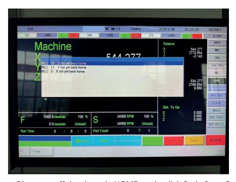
Press F1 to turn off the alarm. In HOME mode, click Cycle Start. Each axis of the machine will automatically return to the mechanical origin, and the machine tool will immediately start the zero return operation. After the zero return is completed, the processing operation can be carried out.
