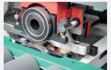
Trimming unit adjustment through the counter convenience and quickly
