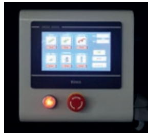
Control panel with 7" touch screen
