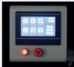
Control panel with 7" touch screen
