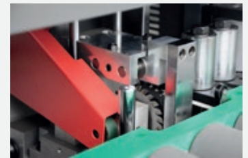
End cutting :Single motor for the automatic end cutting
