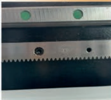
High-Quality Square Rails of Approximately 1 Inch
