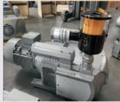
15HP Dry Type Vacuum Pump
